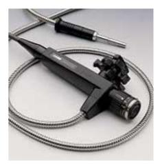
Also incorporated in the viewing piece are four way angulation's controls that allow the steering of the inspection end of the fibre optic cable. A 50mm length at the end of the fibre optic cable can be steered to allow viewing over a hemispherical arc and with an appropriate camera photographs of the object under inspection can be taken as well.
