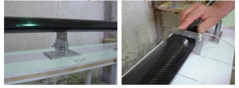
Knife edge used to check the centre of gravity position. It is positioned at the centre of gravity limit (usually only a minimum distance from the heel) and the mast tip should touch down when the mast is placed on the edge. Go/no go gages or calipers may be used to check the cross sections.
