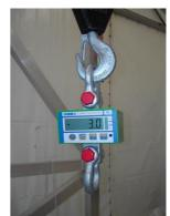
Electronic scales with digital readouts are ideal but should always be calibrated before use. For weighing dinghies a steelyard beam scale is accurate but a spring scale is normally satisfactory. For weighing keel boats, load cells are very accurate, but should be calibrated (twist problems). Alternatively dial reading beam scales can be used.
