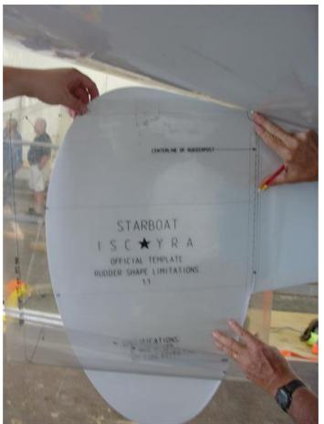
Figure E.1.7 *Profile check with mylar template.*
