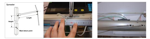
If there is a spreader cut-out, a reference point should be marked on the table before the cut to serve as a spreader height datum. Rigging height marks should be extended to be visible both from the fore and aft edges of the spar.
