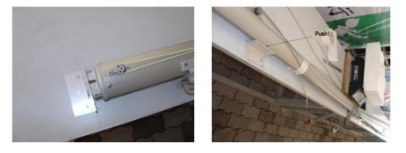
The mast heel must be pushed and kept firmly against the heel stopper. In this example the heel point is also the datum point. The spar has to be also kept tightly against the two stoppers on the mast reference line.
