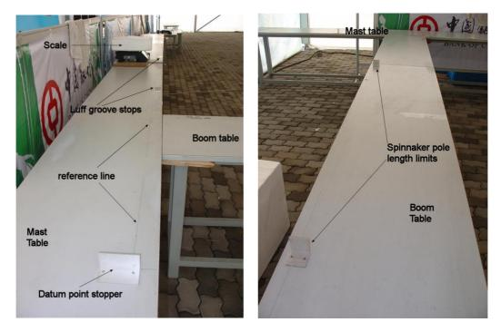
Mast and boom table layout: A strong fitting fixed securely on the table is required for setting the mast heel especially if this is the datum point. Whatever system is used, its mast heel bearing surface should be vertical and perpendicular to the line of
