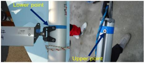
Figure F.2.1 Mast Upper and lower marks and points
