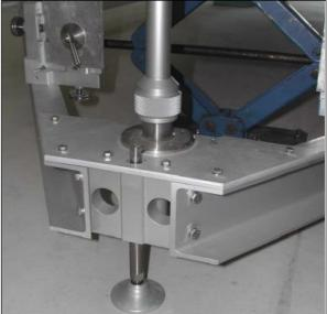
Figure D.1.3.7 Levelling feet
