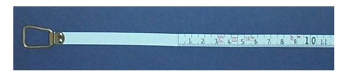
*Figure I.4.1* A measuring tape with an offset zero to eliminate end errors.
