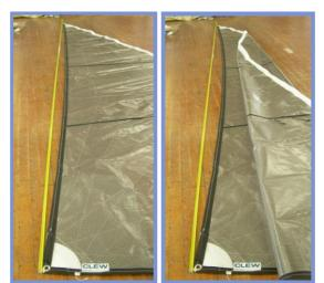
Figures G.2.3.1 & G.2.3.2 Leech flattening before and after flaking.
