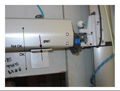
With the boom and mast joined together, the boom position relative to the lower point may be checked: the top surface of the boom (bottom in the picture above) must be at the same height as the lower point or higher. The visible gap in the picture indicates that the boom is improperly positioned.
