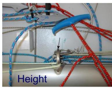
Spinnaker hoist height with the halyard held at 90° to the spar. Spinnaker pole fitting height from the center of the fitting.
