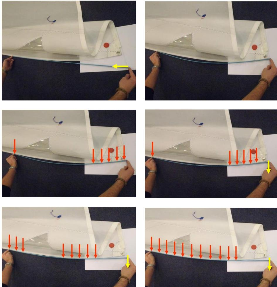
When the line of the extension of the edge is uncertain and not repeatable, leading to inconsistent measurement points, the measurement of the sail should be refused and the certification authority contacted for consultation.
