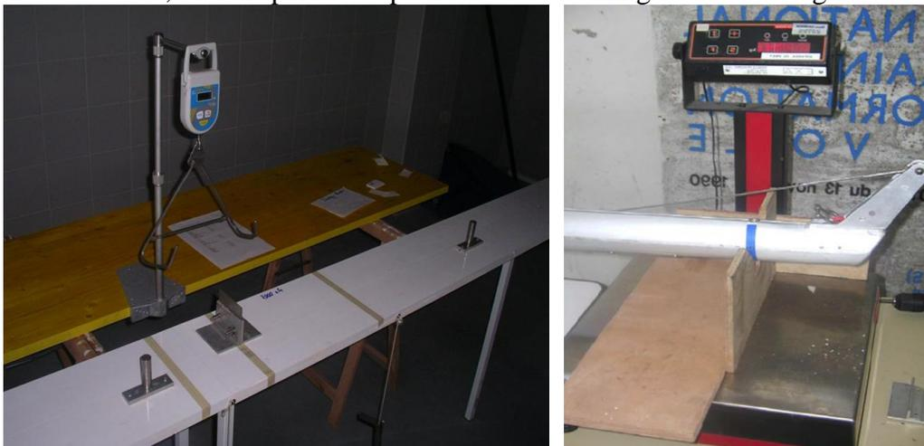
Mast weight / centre of gravity (left) and tip weight (right) measurement. The centre of gravity may be checked using a knife-edge to balance the mast.
