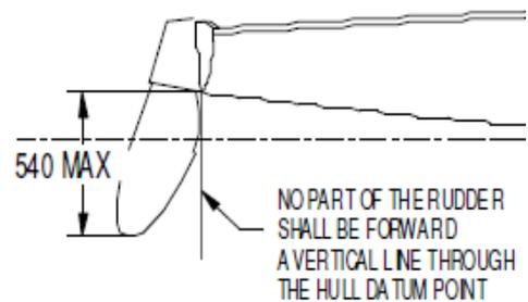
In the example to the right, class rules specify the length of the rudder when positioned on the hull as the minimum distance from the hull underside, the position of the leading edge relative to the Hull datum point, and the angle of the blade by checking the distance from the lowermost point to the HDP.
