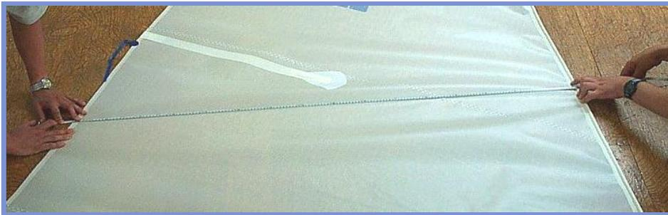
**Figure G.2.3.4** *Proper tensioning of sail for wrinkle removal.*
