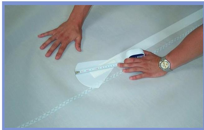
**Figure G.4.3** *Batten pocket patch size.*
