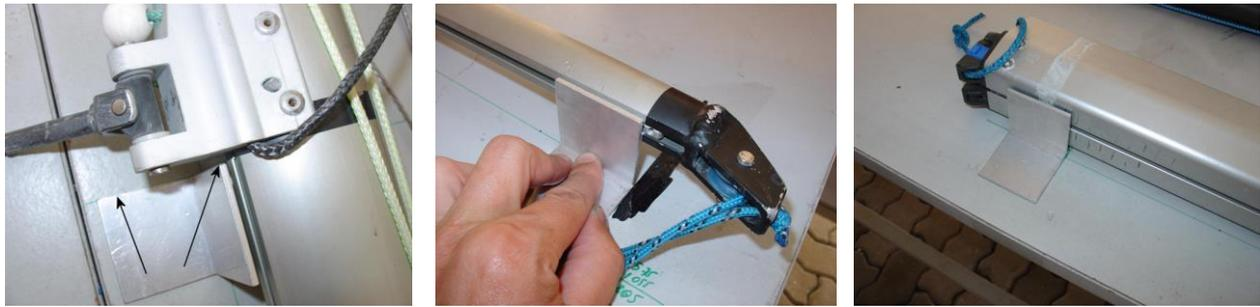
Marks on the table should be projected on the spars with a square, never eye-balled.
