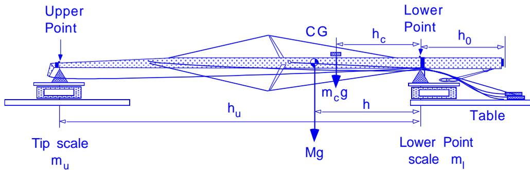
**Figure F.3.3** Simultaneous Tip weight and mast weight measurement, with halyard tails on the lower point scale but turnbuckles supported on the table.
