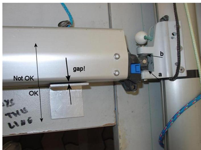
With the boom and mast joined together, the boom position relative to the lower point may be checked: the top surface of the boom (bottom in the picture above) must be at the same height as the lower point or higher. The visible gap in the picture indicates that the boom is improperly positioned.
