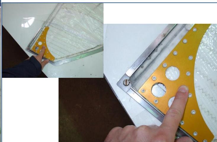
**Figure G.3.2** *Head positioned on jig*
