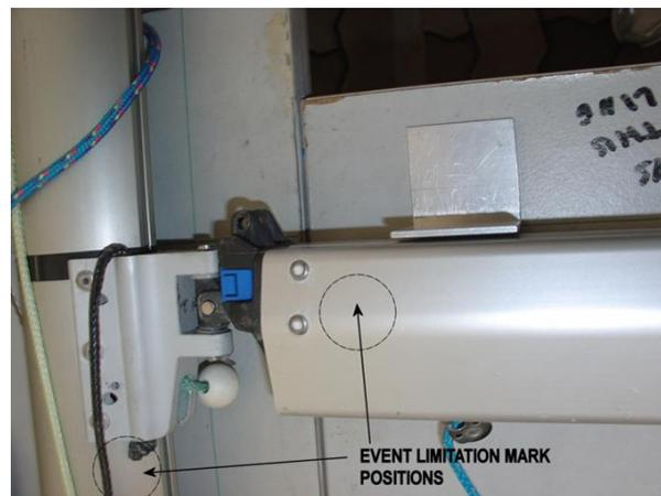
The position of event limitation marks (usually stickers) is also important, because the stickers have to be visible on the water, but also protected from wear and tear. They have to be positioned at the same place on all boats so that the inspectors know where to expect to find them.
