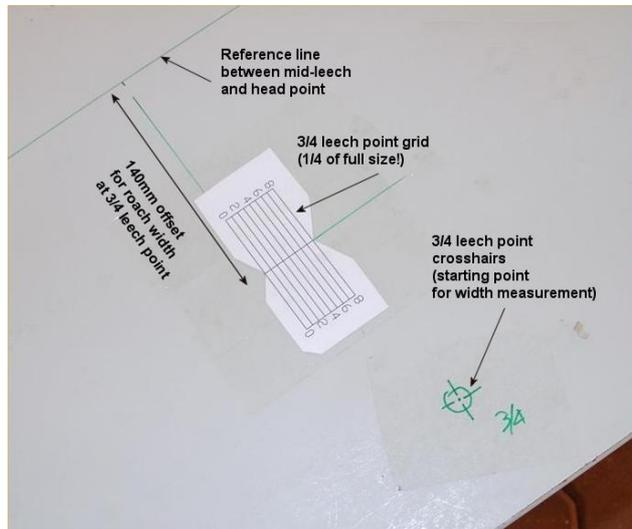
**Figure G.2.4.5** *Three quarter point scale & width datum reference mark*
