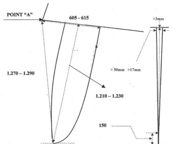
Similarly, keel fore and aft position may be controlled from the HDP, and depth from the keel line at certain stations. In some cases, this may be conveniently done with purpose made gauges as shown below.
