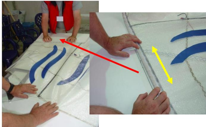
**Figure K.3.2.4** *Sail width measurement on sail table with marks*
