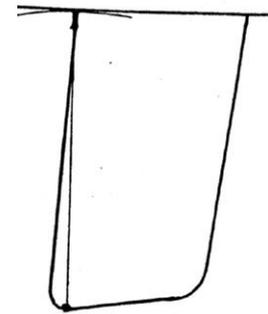
The depth of the rudder blade below the hull is normally taken in the same manner. It is -unless otherwise indicated in the class rules- the vertical distance below the lowest point of the transom, which means that the hull must be also properly levelled before.
