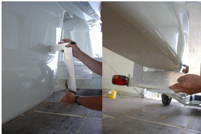
**Figure E.2.6** *Thickness control.*
