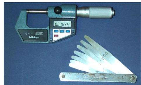
A set of standard feeler gauges are also required when checking sail ply thickness.
