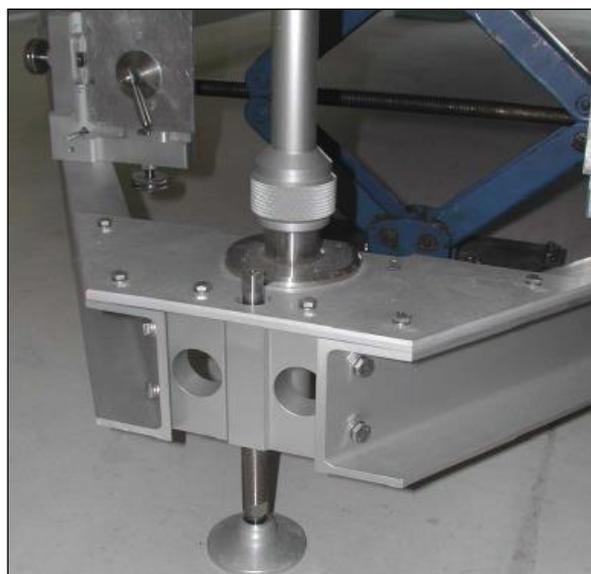
**Figure D.1.3.7** *Levelling feet*
