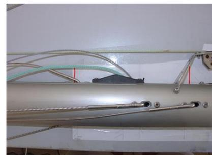
If there is a spreader cut-out, a reference point should be marked on the table before the cut to serve as a spreader height datum. Rigging height marks should be extended to be visible both from the fore and aft edges of the spar.
