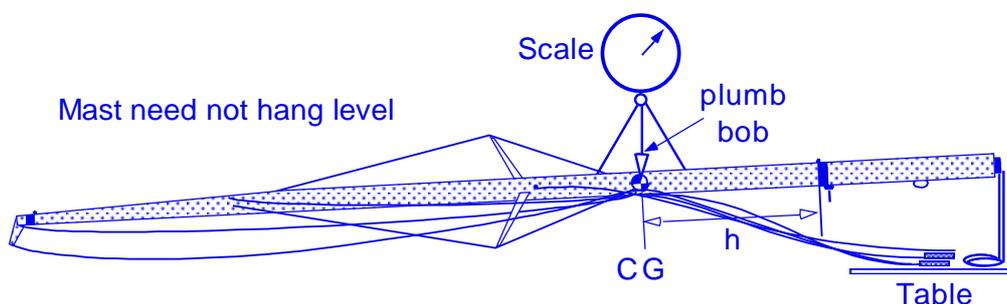
**Figure F.3.2** Larger masts can be weighed using a hanging scale, and the CG height determined simultaneously with a plumb bob. Note that the mast need not be precisely horizontal as the CG is always directly under the free suspension point.
