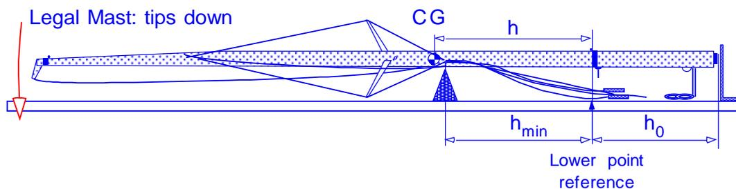
**Figure F.3.1** Determination of the mast CG by balancing on a knife edge. For regatta inspection the knife edge is set at the minimum permitted distance from the datum point and the mast tip must go down when released.
