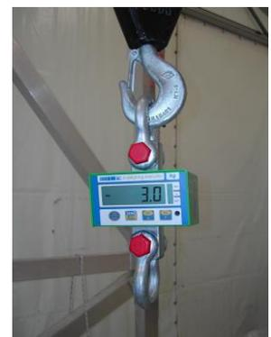
Electronic scales with digital readouts are ideal but should always be calibrated before use. For weighing dinghies a steelyard beam scale is accurate but a spring scale is normally satisfactory. For weighing keel boats, load cells are very accurate, but should be calibrated (twist problems). Alternatively dial reading beam scales can be used.
