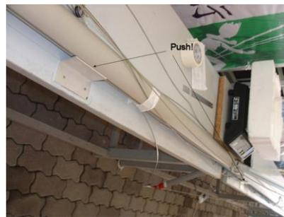
The mast heel must be pushed and kept firmly against the heel stopper. In this example the heel point is also the datum point. The spar has to be also kept tightly against the two stoppers on the mast reference line.
