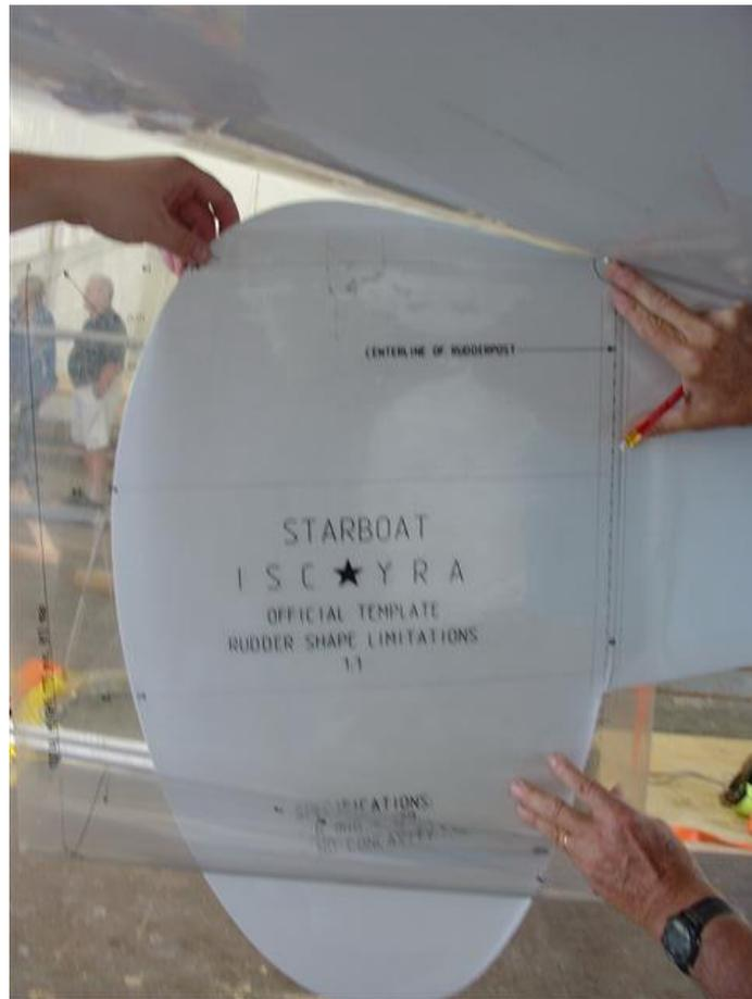
**Figure E.1.7** Profile check with mylar template.
