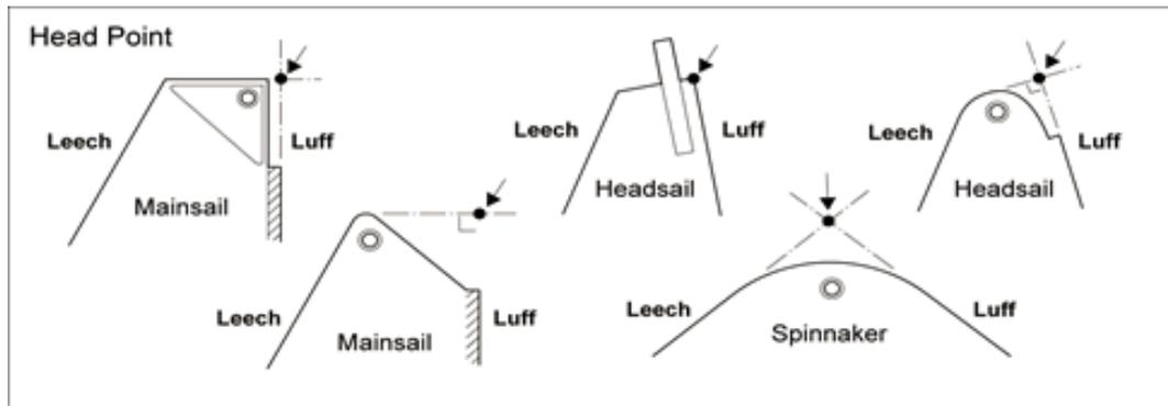
The head point on a mainsail is the intersection of the luff, extended as necessary, and the line through the highest point of the sail at 90° to the luff. In this case, any attachments are to be included (Figure G.2.1.9)
