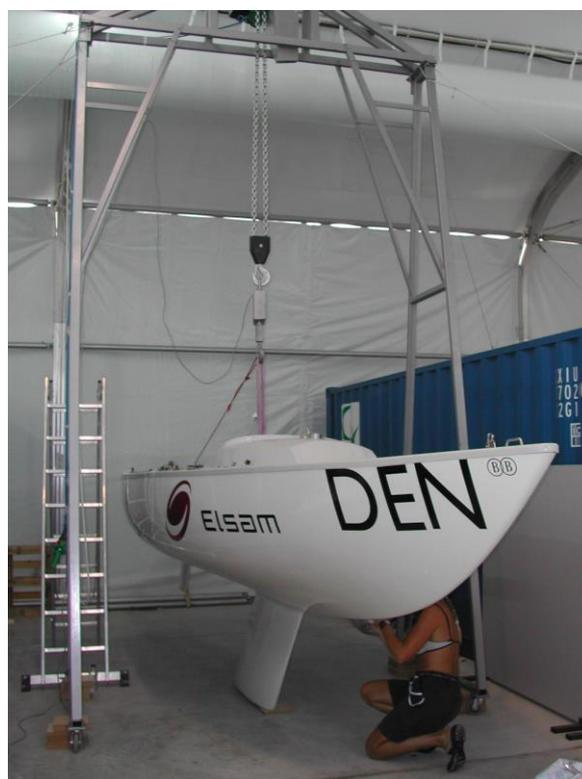
The weighing machine has to have adequate capacity and preferably should be operating within about the range of one-half to three-quarters of its capacity.
