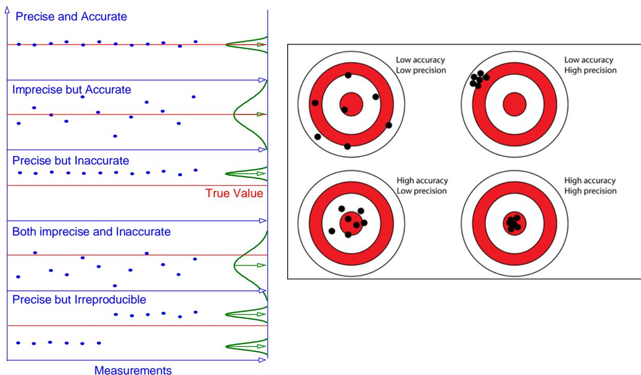
**Figure 1.3.1** Histograms of the scatter of many measurements of the same quantity illustrating the difference between accuracy, precision and reproducibility.
