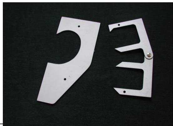
curvature of the hull and projects the curve up to the sheerline. However, it should be noted that this device assumes the topsides to be a circular curve, and if it is not then an error will occur. To overcome this point in one-design classes with curved topsides C-templates can be made for each measurement station using the lines plan, or preferably full size sections of the hull.
