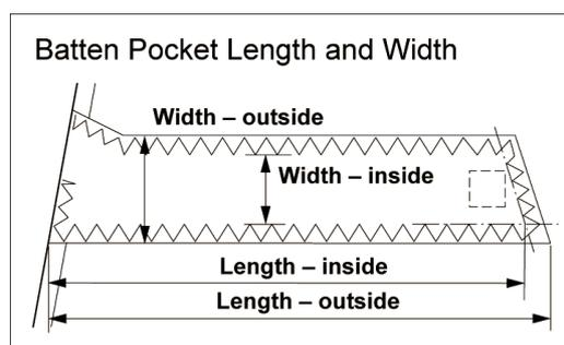
**Figure G.4.4** *Batten pocket length and width measurement.*
