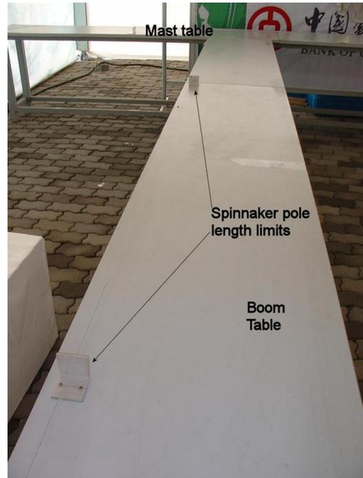
Mast and boom table layout: A strong fitting fixed securely on the table is required for setting the mast heel especially if this is the datum point. Whatever system is used, its mast heel bearing surface should be vertical and perpendicular to the line of measurement.
