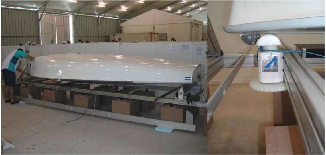
Figure D.1.3.3 Spanish 470 Jig with a hull on top (left) and the modular framing and levelling screws detail (right)
