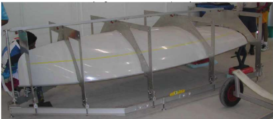
Figure D.1.3.5 The Europe hull inside the jig levelled and aligned using car jacks
