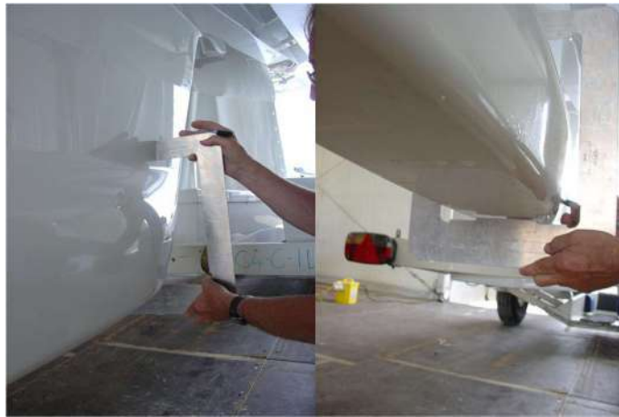
Figure E.2.6 Thickness control.
