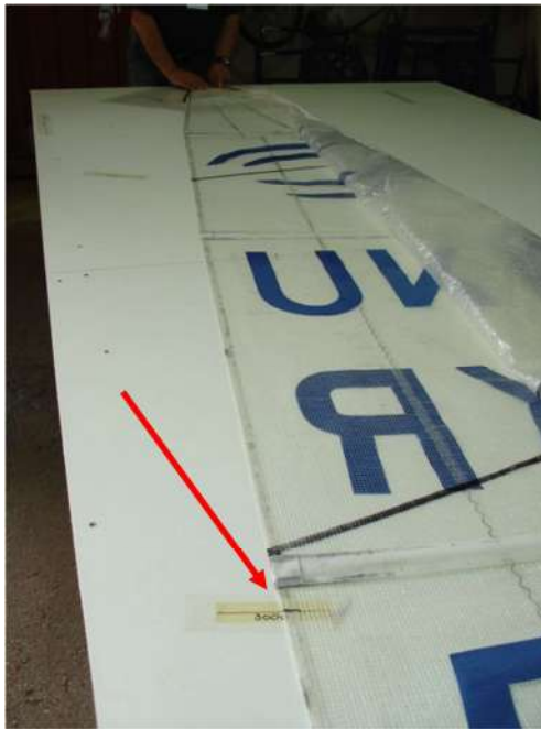
Figure G.3.3 Radial distance leech point mark
