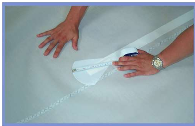
Figure G.4.3 Batten pocket patch size.
