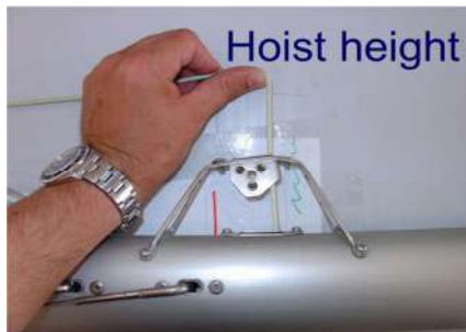
Spinnaker hoist height (left) with the halyard held at 90° to the spar. Spinnaker pole fitting height (right) from the center of the fitting.
