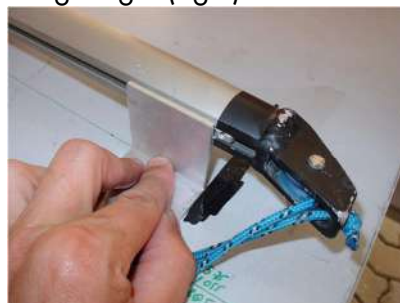
Spinnaker hoist height (left) with the halyard held at 90° to the spar. Spinnaker pole fitting height (right) from the center of the fitting.
