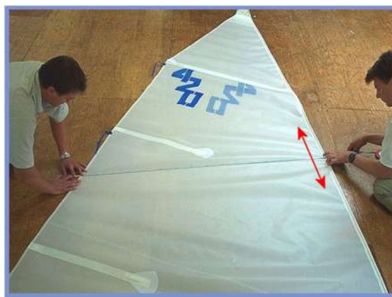
Figure K.3.2.4 Sail width measurement with measurement tape
