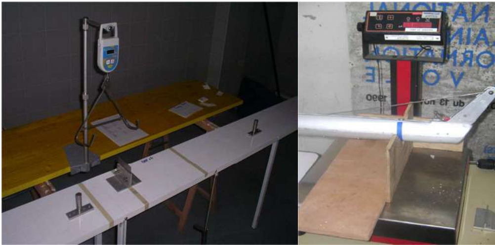
Figure F.3.2 Mast weight / centre of gravity (left) and tip weight (right) measurement. The centre of gravity may be checked using a knife-edge to balance the mast.
