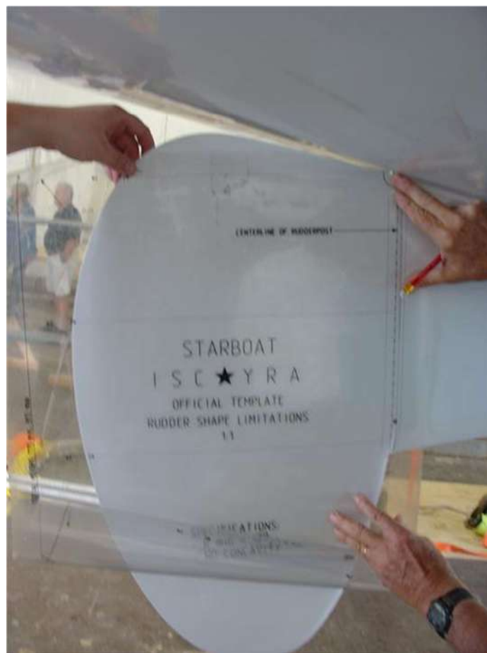
Figure E.1.7 Profile check with mylar template.
