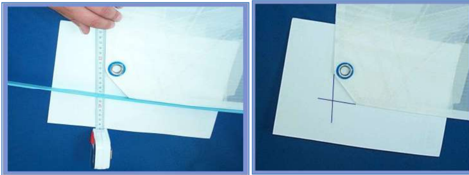
Figure G.2.1.7 Clew point: sail edge extensions marked on paper.
